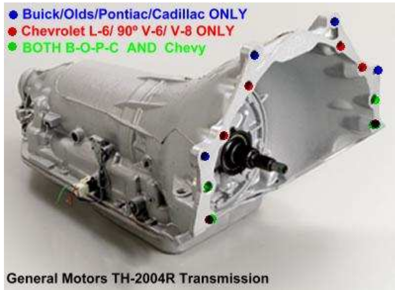
Photo of a 200-4R transmission with BOP design bell housing bolt pattern. Notice the valley between the top two bolt holes.
