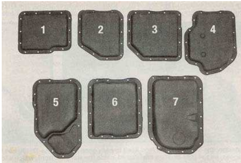
Transmission identification by pan shape with gear ratios.
